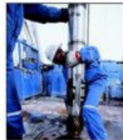
Preparation of the drill bit and of the guidance system
