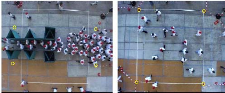
Figure 1 Examples of pedestrian experiments; a) narrow bottleneck experiment, and b) four-directional crossing flow experiment. Yellow circles (and demarcation on the floor) indicate the respective walking areas. The figure also shows the so-called pincushion distortion and the slight rotation of the camera (around 1%).
